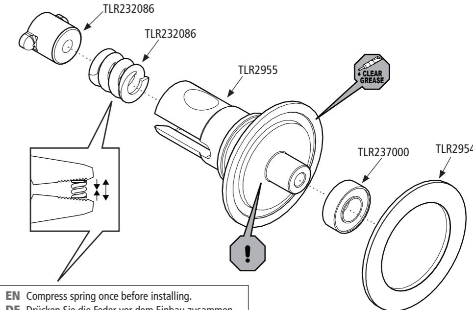
EN Compress spring once before installing.
